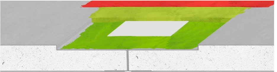
Fig. 5. Filling in joints between PRO type edges with utilisation of fliseline, or paper tape
