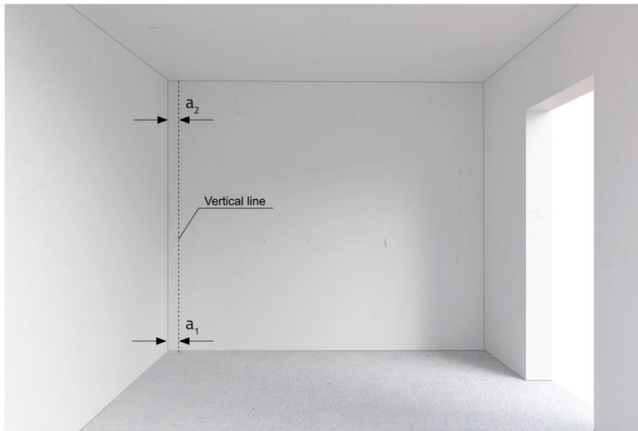
Fig. 12. The manner of taking measurements – deviations of surfaces from the vertical direction
