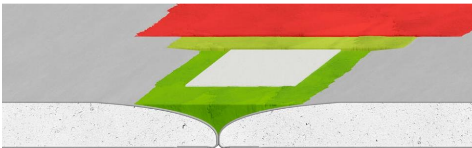
Fig. 7. Filling in joints between KPOS type edges with paper or glass fibre tape embedded in joint filler compound
