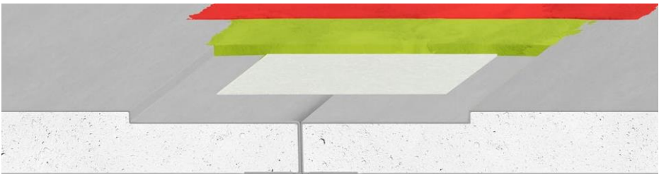
Fig. 3. Filling in joints between PRO type edges with utilisation of self-adhesive tape
